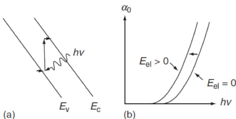
(a) electric field tilts the band structure. When a valence electron absorbs a photon, it tunnels into the conduction band. (b) A red shift is observed.
