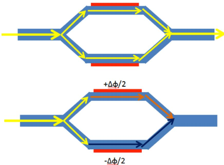
Left - Mach-Zehnder modulator operation: electrical field changes the refraction index of the material being able to create destructive interference
