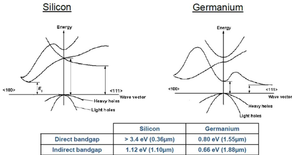
Left - Comparison of Silicon and Germanium band structures[3]
