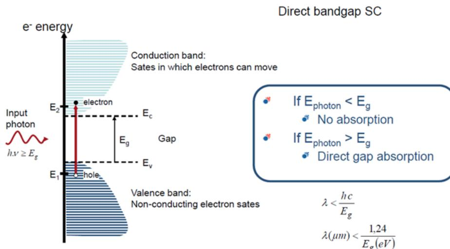
Left - Absorption in direct bandgap semiconductors[3]
